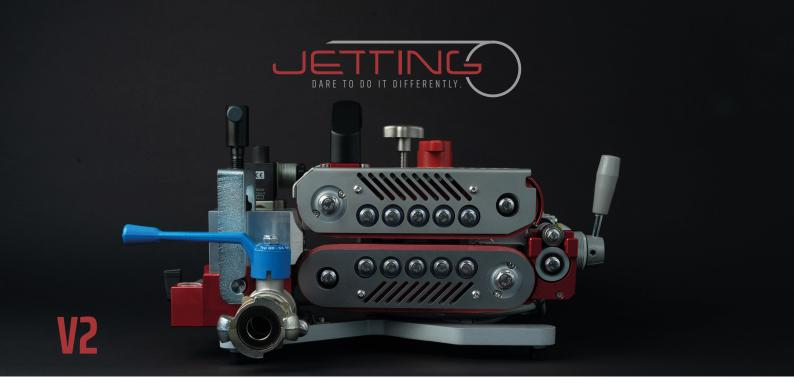
Robust and compact pneumatic operated fiber blowing machine with the unique Joystick controller securing optimal control of the installation. This machine can be configurated from 2,4 to 16 mm cable and 7 to 50 mm duct. Anodized aluminum construction makes this machine both lightweight and easy to maintain.
