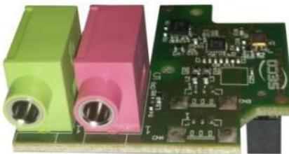
For the Qseven® modules offering I2S Audio interface, it is possible to use an I2S Audio adapter module, which can be mounted directly on carrier board's connector CN28 (piggyback connection).
