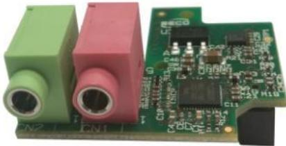
According to the Qseven® standard, the Qseven® modules can implement HD Audio, AC'97 or I2S Audio interface. For this reason, the CQ7-A42 carrier board doesn't have any audio codec onboard, and it is therefore not able to offer directly a PC-like audio interface.
