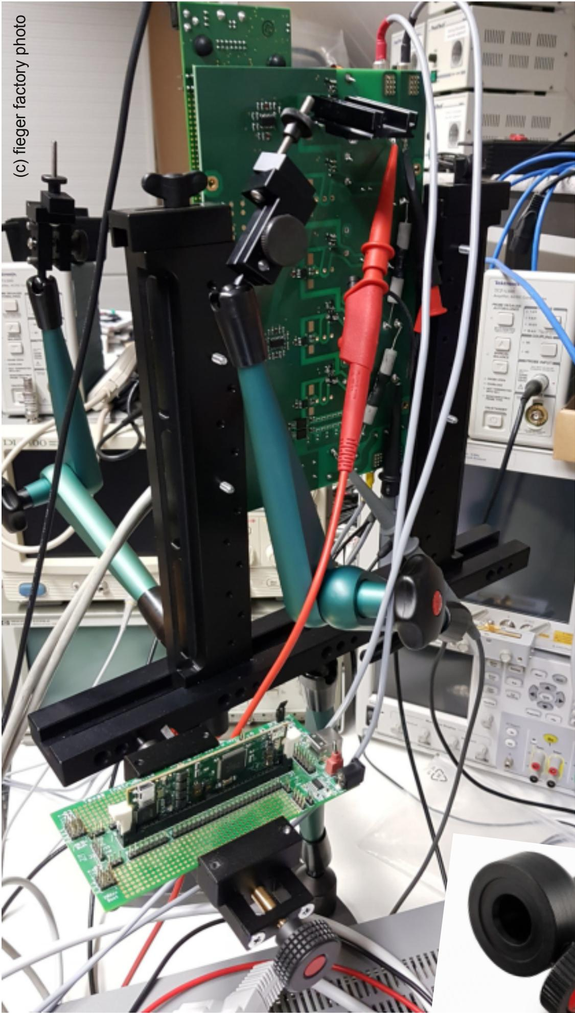
The vice mounted on the ClampMan using an additional base adapter "104500"
