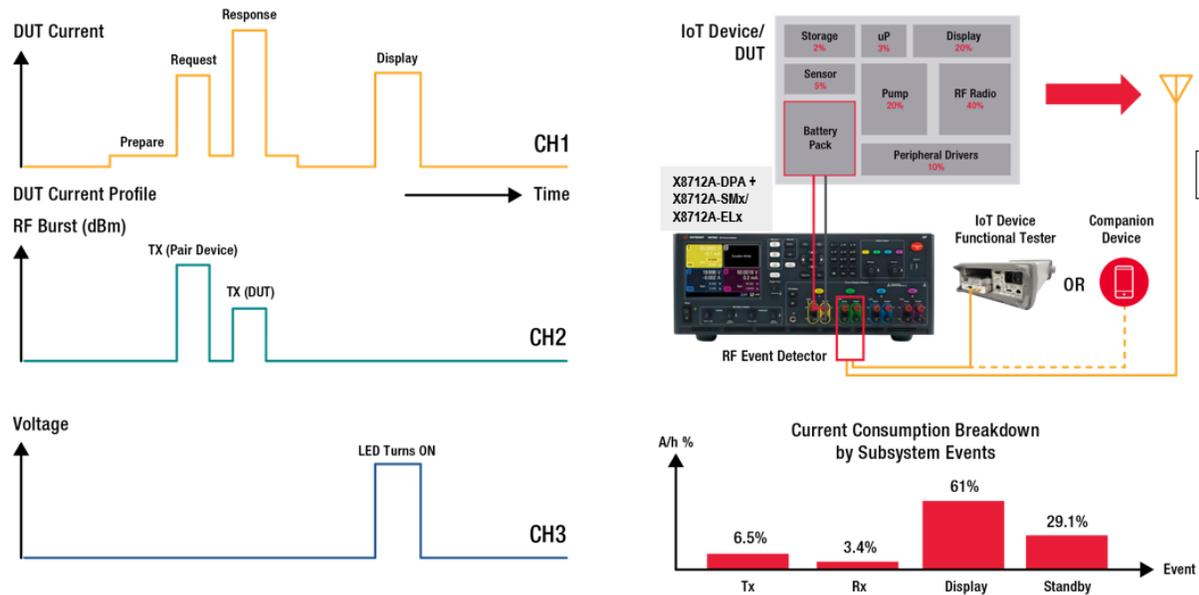
Figure 2. The X8712A Event-based Power Analysis Concept
