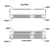
The connector is CN6, which is a standard 52pin miniPCI Express connector, type MMT p/n MINIPCIE6001-Rt52GF, H=4mm, with the pinout shown in the table on the left.
